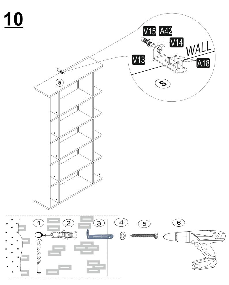
Check the Wall type before installation of dowel. Wall is drilled with equal diameter of dowel.(08mm) Universal Plastic Dowel provides the general purpose usage. Requires two stages assembly.
